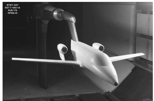
Fig. 15 Photograph of \frac{1}{8} -scale model installed in Boeing Transonic Wind Tunnel (BTWT).
