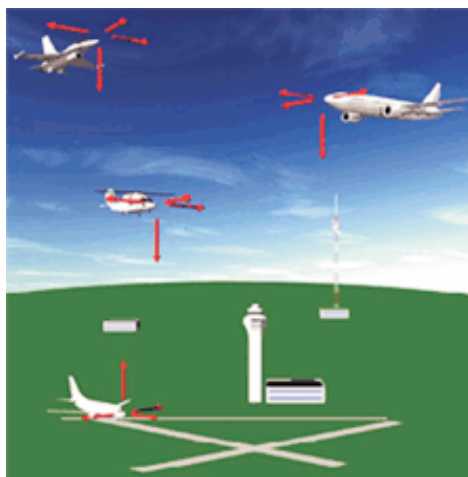
FAA depiction of aircraft communicating at different altitudes via ADS-B.
